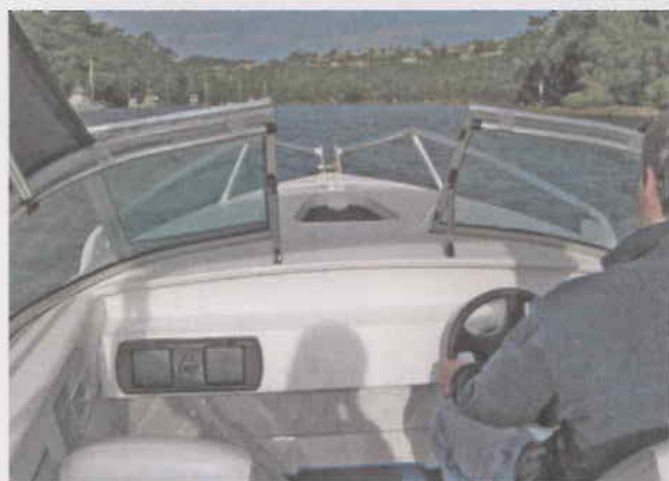
Left: The Bay Cruiser's windscreen rail is high enough to be out of the skipper's line of sight. Right: A drop down rear lounge makes a lot of sense in a smaller fishing boat; with the lounge dropped there's even more room.
